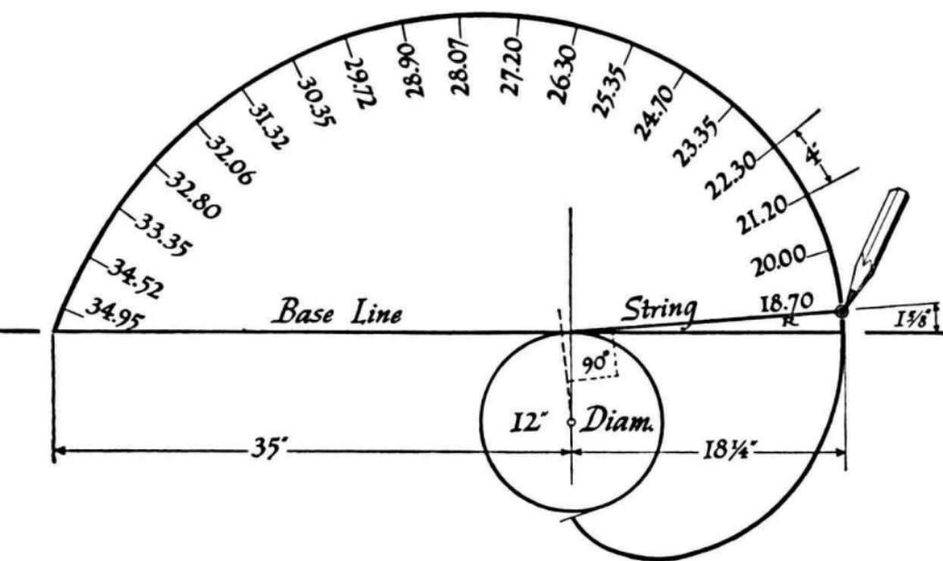
The above drawing shows the layout of an involute derived from a twelve-inch cylinder, which experience has shown to be a satisfactory size.
