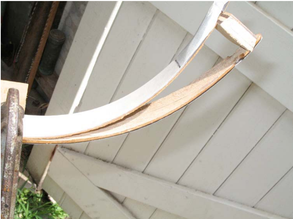
Figure 5 - The delaminated limb protected with masking tape on the glass surfaces, a clamp preventing extension of the delamination while the limb halves are kept open for examination and preparation for gluing.
