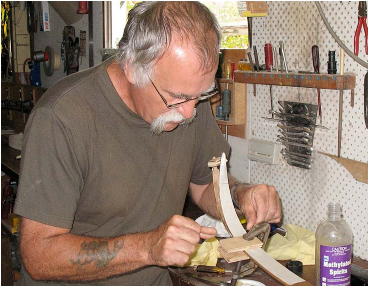
Figure 7 - Dave Keable working glue into joint using a wire thread. Note that the joint is clamped to prevent further splitting of the delamination while it is being worked on.
