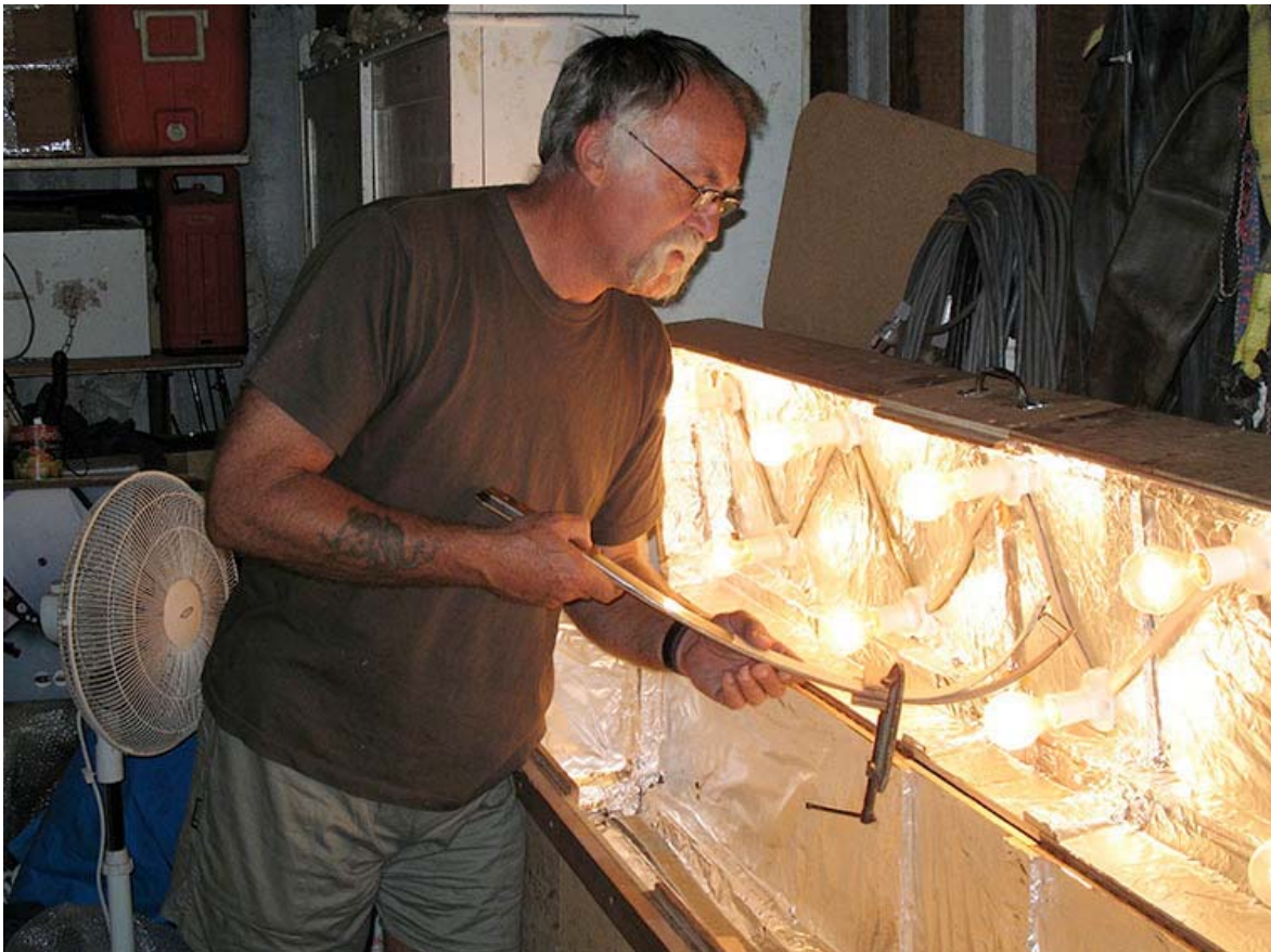
Figure 6 – Dave Keable warming the open glue joint in the lid of the hot box before gluing.
