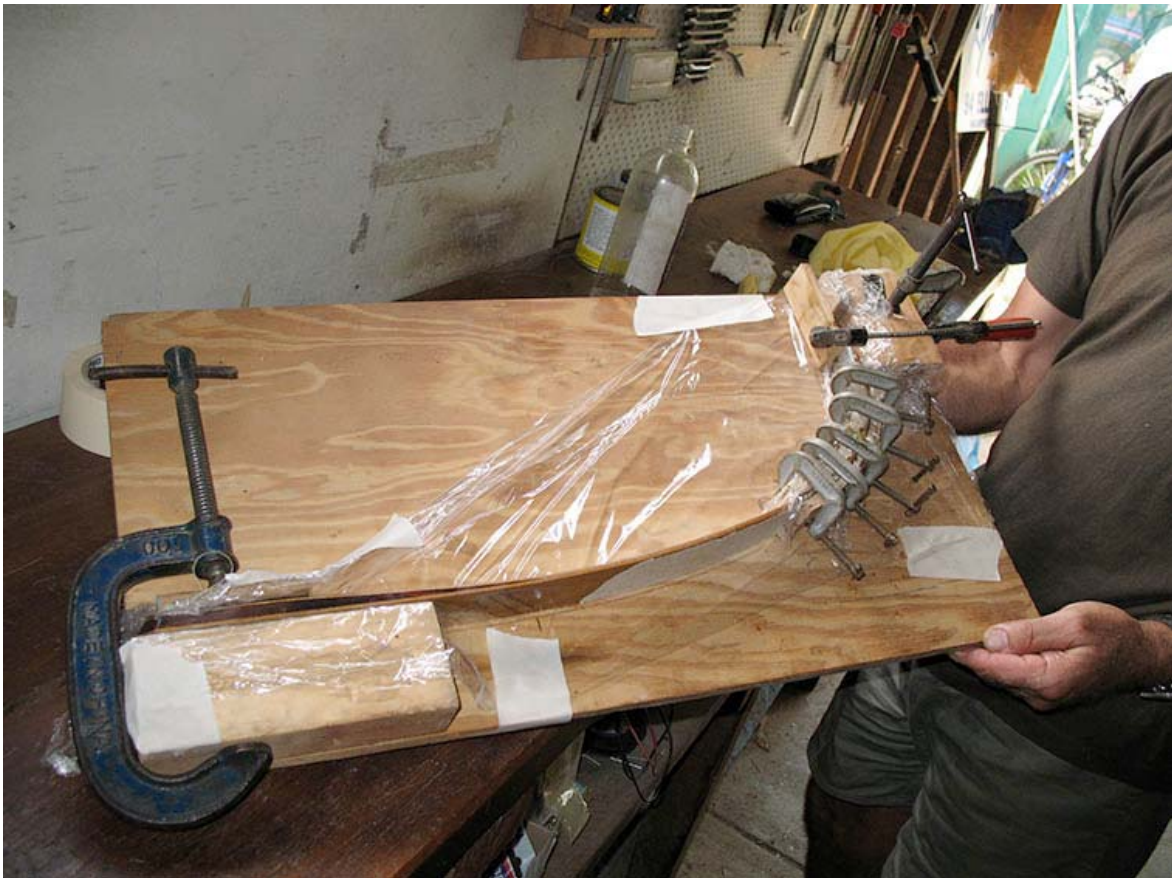
Figure 4 - The jig in operation. The placement of the various clamps, Glad Wrap and masking tape on the limb can clearly be seen. At this stage, it is ready for the oven.
