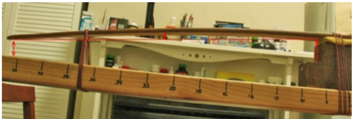
7. Pic showing mid-point of the bent limb between the 20" and 22" markers being deepest point of curvature of limb. The vertical distance at the limb tip is the required amount of bend.
