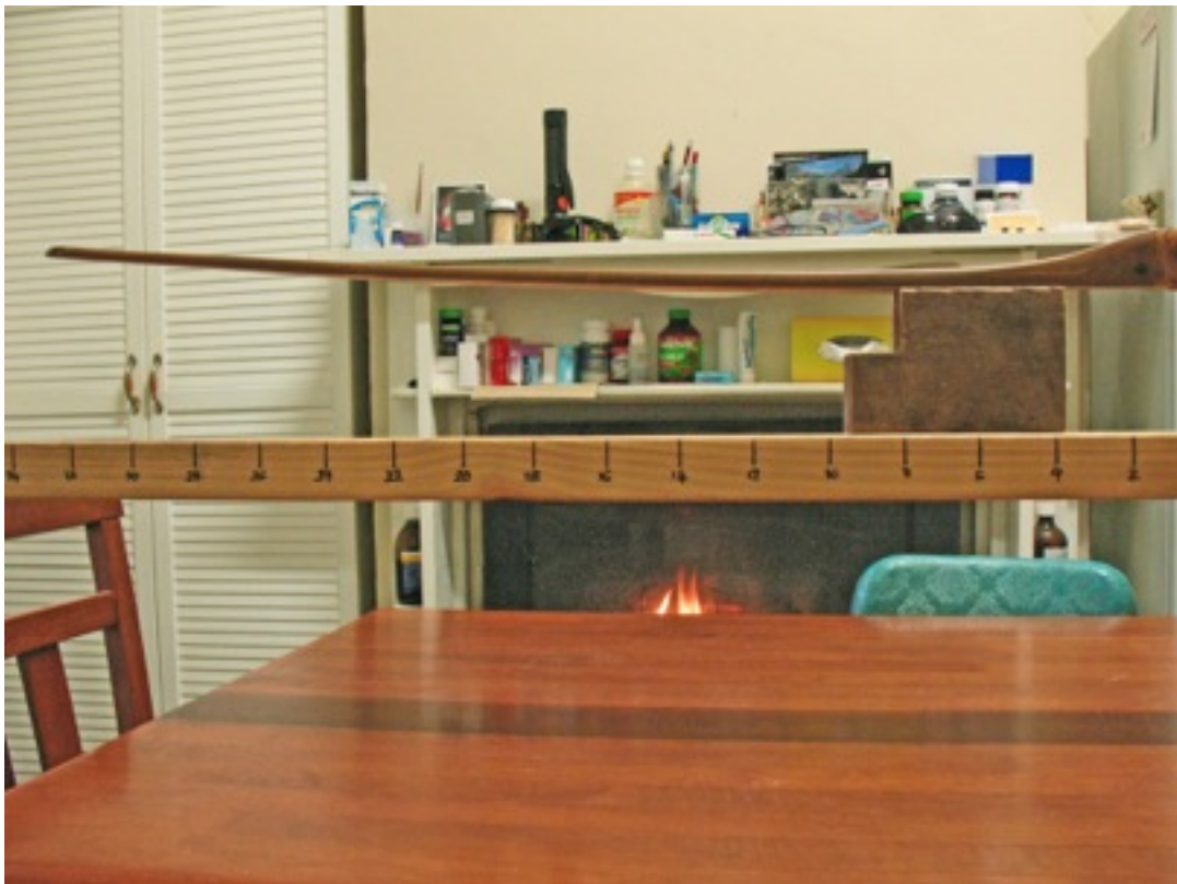
4. The amount of unsupported limb at each end of the mounting blocks must be of equal length; in this case 25" to the limb nock at each end.
