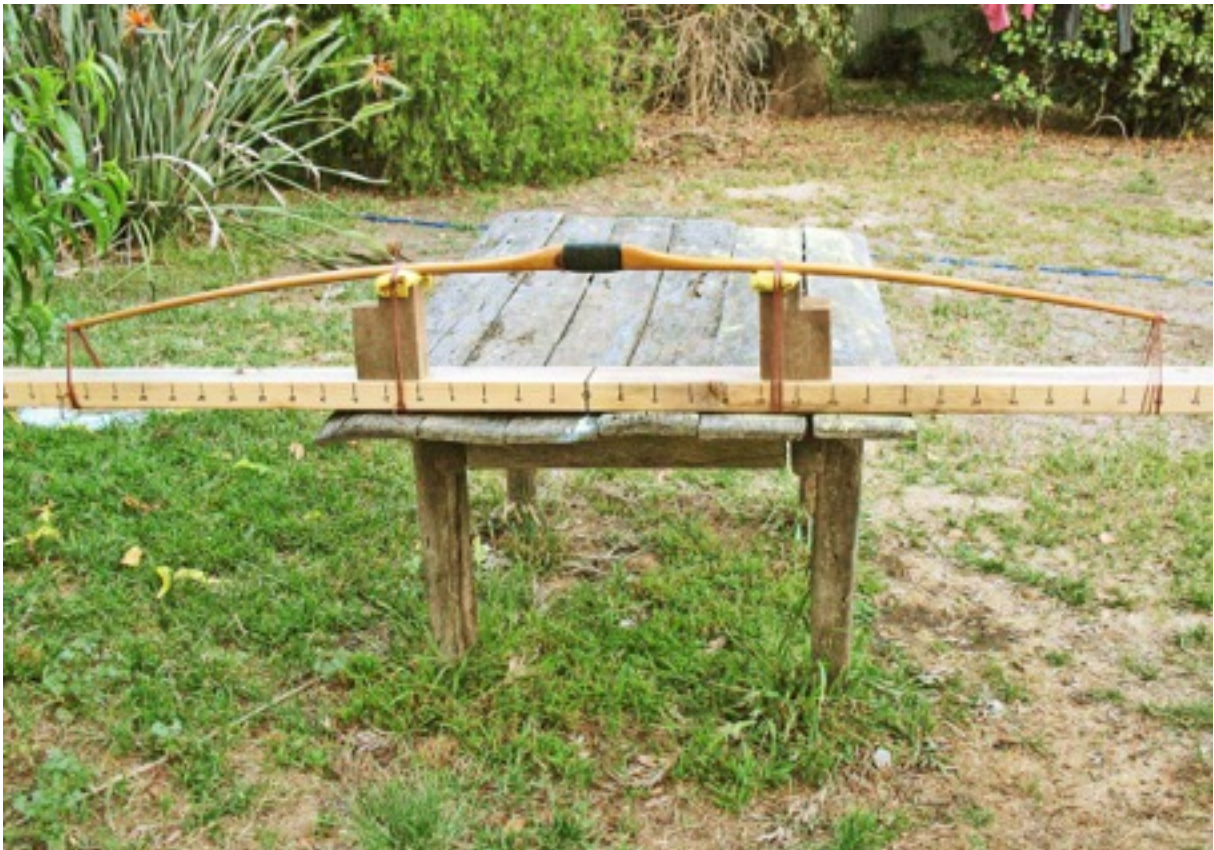
2. 1940s Ben Pearson 7056 Lemonwood fibre-backed target bow mounted on bending jig.
