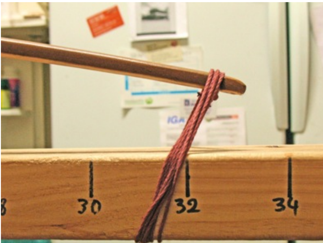
6. Limb tip lashed and drawn down by required amount of bend to 3.5cm above base.
