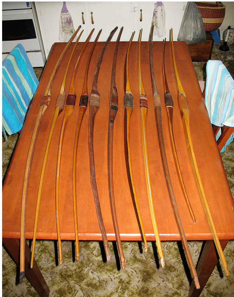
1. Ten bows from my collection showing varying degrees of set. The bow fifth from the left has just over 4 inches of set.
