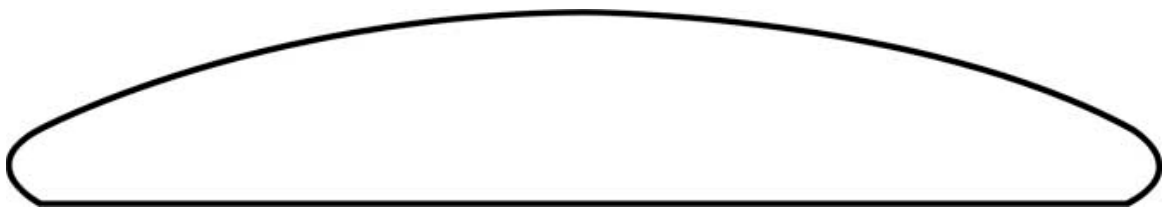
Figure 3: Cambered limb section of Holmegaard log bow.
