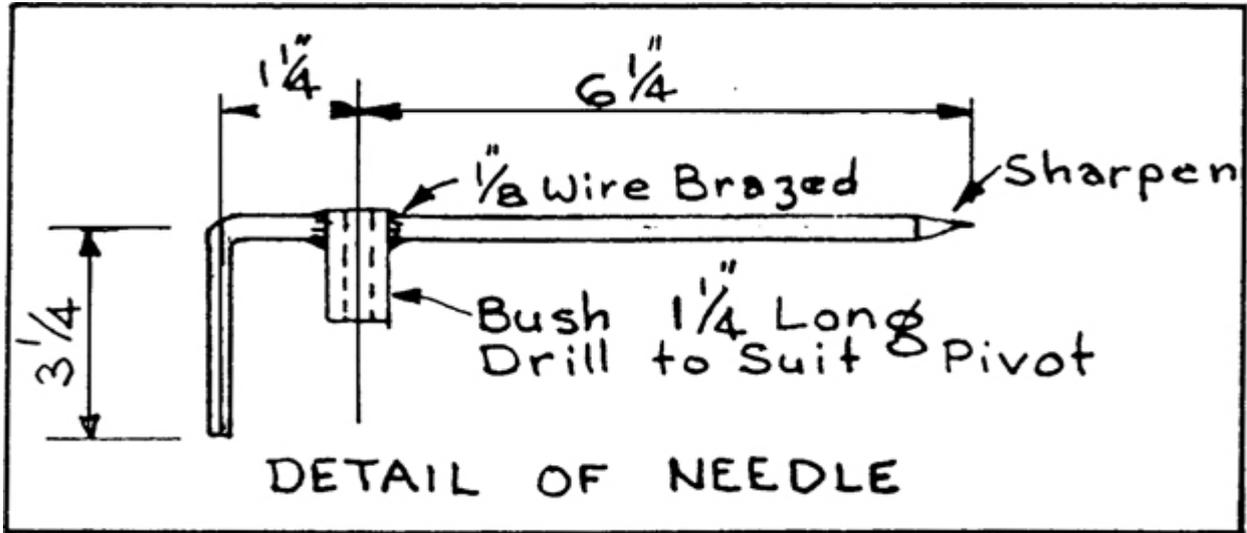
The position of the pivot pin is critical and must be placed as shown in the detail below. Care must be taken to ensure that the pivot pin protrudes from the back face of the jig horizontal and at right angles to the surface.
