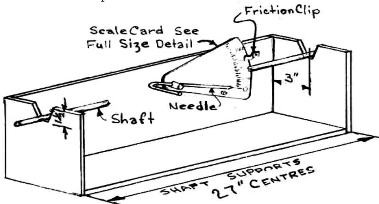
SHAFT supports are simple notches cut in the two end walls of the jig. The horizontal surface at the bottom of the notches should be filed to a rounded edge so that the shaft is suspended at a point rather than on a flat area. It is important that shaft supports are at exactly 27" centres<sup>1</sup>.
